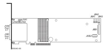
Note: Connectors J6A1, J6A2, and J6A3 are behind the LSIiBBU07 when the iBBU is installed, but they are still accessible.
